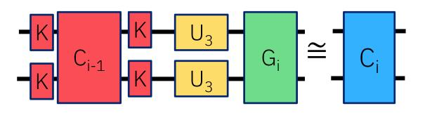
finalize decomposition by solving for the interleaving single-qubit gates.
